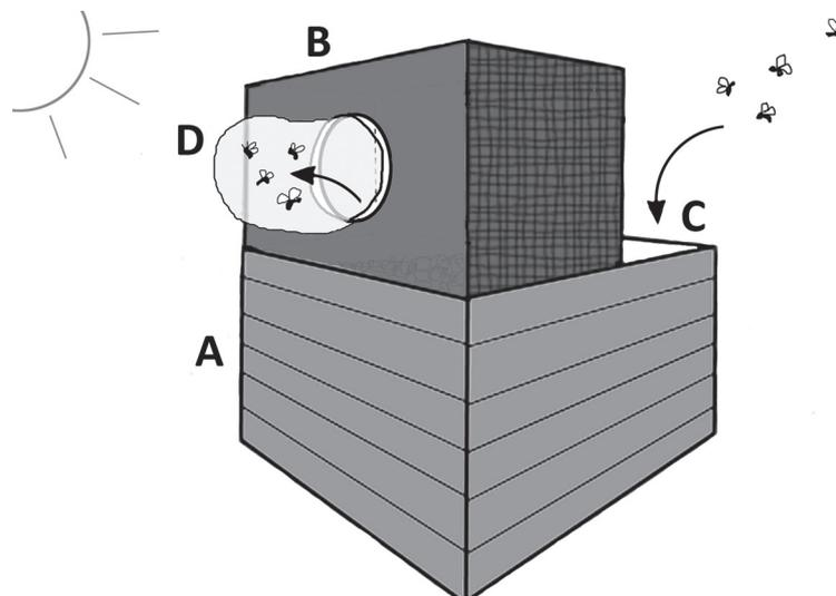
**Figure 1.** Setup used collecting arthropods leaving a composter. (A) Composter, (B) Acrylic glass cage, all sides covered with fly screens and black plastic sheets. The cage used in the experiments had two openings for collecting arthropods, but for clarification only one opening is illustrated, (C) Opening between the composter and the cage through which arthropods could enter the composter, (D) plastic bag for collecting arthropods.
